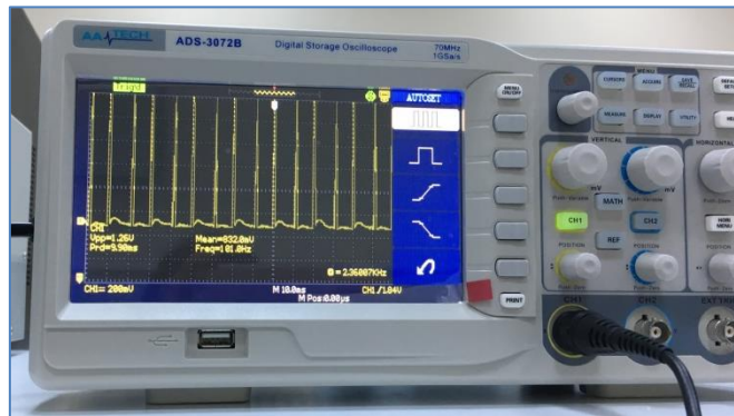
Figure 5. ECG signal is displayed as seen in the oscilloscope
